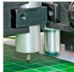
1. Dual tool head delivers class-leading force to both the crease and cut tools
