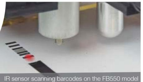
IR sensor scanning barcodes on the FB550 model
