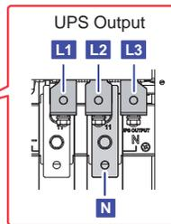
(Figure 2-9: Wiring Terminals\_ UPS Output)
