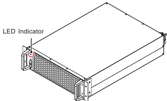
(Figure 5-36: STS Module's LED Indicator)
