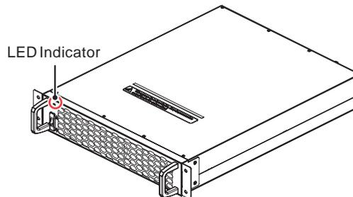
(Figure 5-48: Power Module's LED Indicator)
