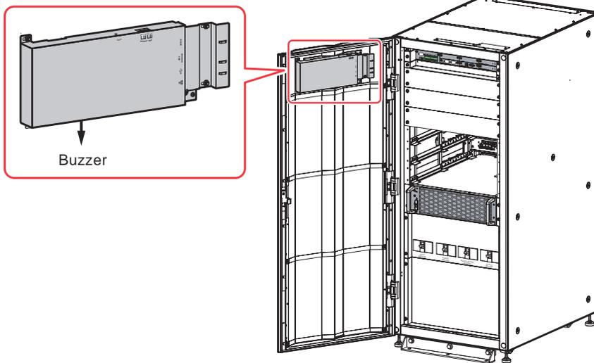
(Figure 2-13: Buzzer Location)
