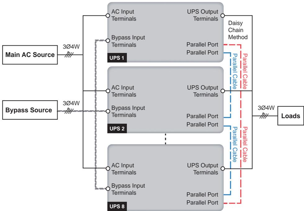
**(Figure 5-19: Parallel Units Dual Input Wiring Diagram)**
