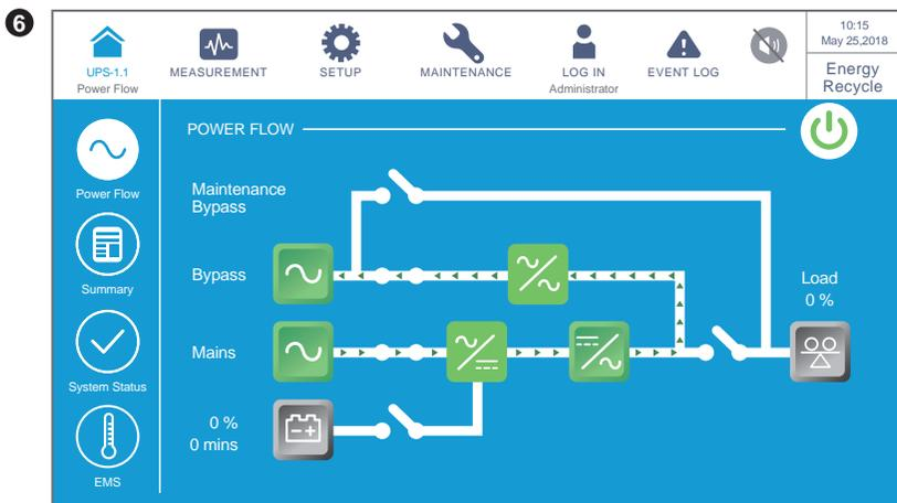
The screen above indicates that the UPS is in **Energy Recycle** mode. The output power will be recycled to the main input without being sent to the loads and the aging test could be conducted. For **Energy Recycle** mode settings, please refer to **7.10.2 Mode Setting** and **6.2.8 Energy Recycle Mode Start-up Procedures**.
