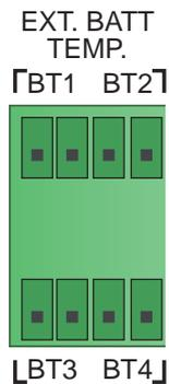
(Figure 4-7: External Battery Temperature Dry Contacts Design)
