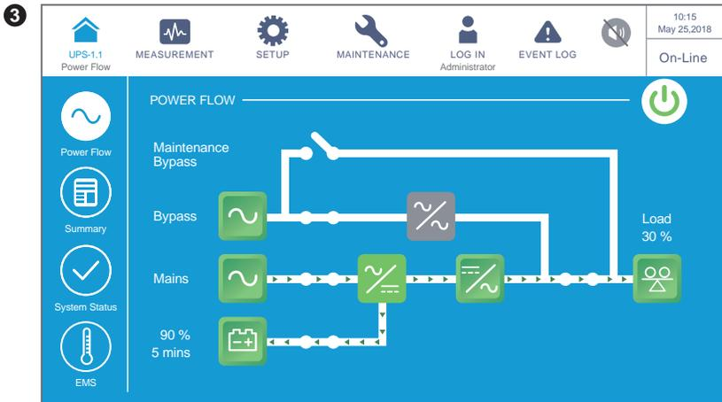
The screen above indicates that the UPS is in **On-Line** mode, and power supply of the loads comes from the inverter. Please refer to **7.10.2 Mode Setting** and **6.2.1 Online Mode Start-up Procedures**.
