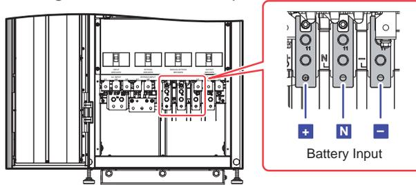
(Figure 5-9: Wiring Terminals\_ Battery Input)
