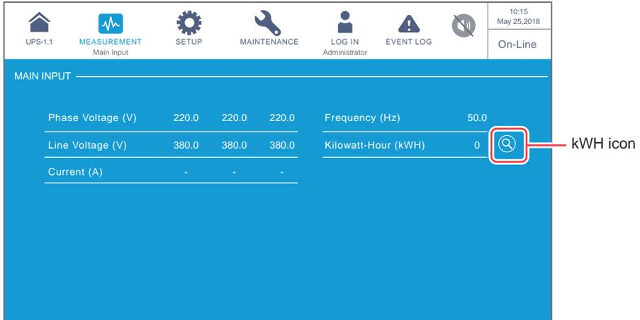
Tap the KWH icon (
