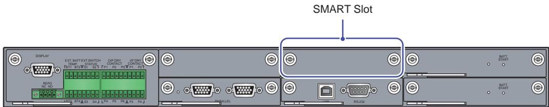
(Figure 4-15: SMART Slot Location)
