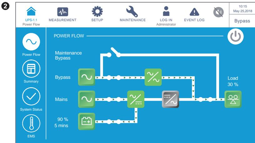
The screen above indicates that the UPS is in **Bypass** mode and the inverter is off.
