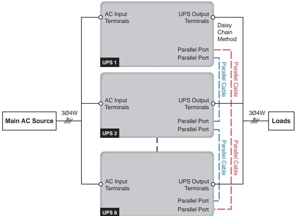
(Figure 5-17: Parallel Units Single Input Wiring Diagram)
