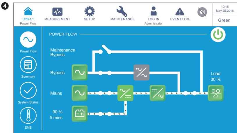
The screen above indicates that the UPS is in **Green** mode, and power supply of the loads comes from the inverter. Power modules will take turn to rest depending on the total load situation. For **Green** mode settings, please refer to **7.10.2 Mode Setting** and **6.2.7 Green Mode Start-up Procedures**.
