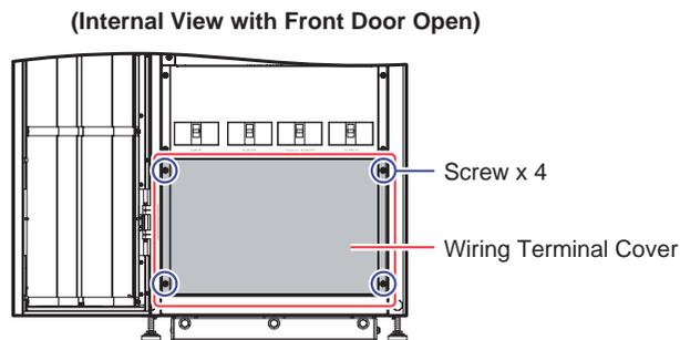
(Figure 5-5: Wiring Terminal Cover & Screw Location)
