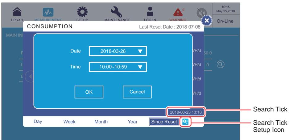
Tap 'OK' to complete the setup for Search Tick, and you will see the date and time in the lower right corner of the window. After that, select and tap one of the kWh Statistics Sheet Tabs to view the column chart of different time scales (Day/ Week/ Month/ Year/ Since Reset).
