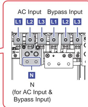
(Figure 5-6: Wiring Terminals\_ AC Input & Bypass Input)
