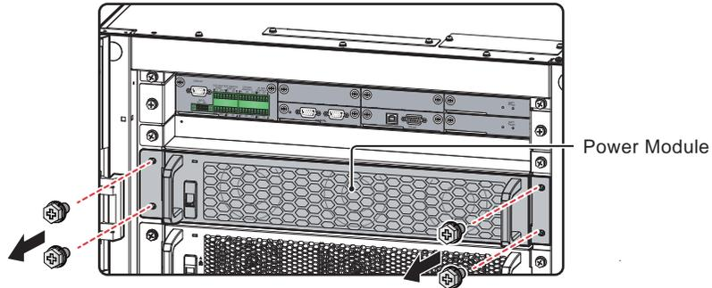
(Figure 5-45: Remove the Four Screws)
