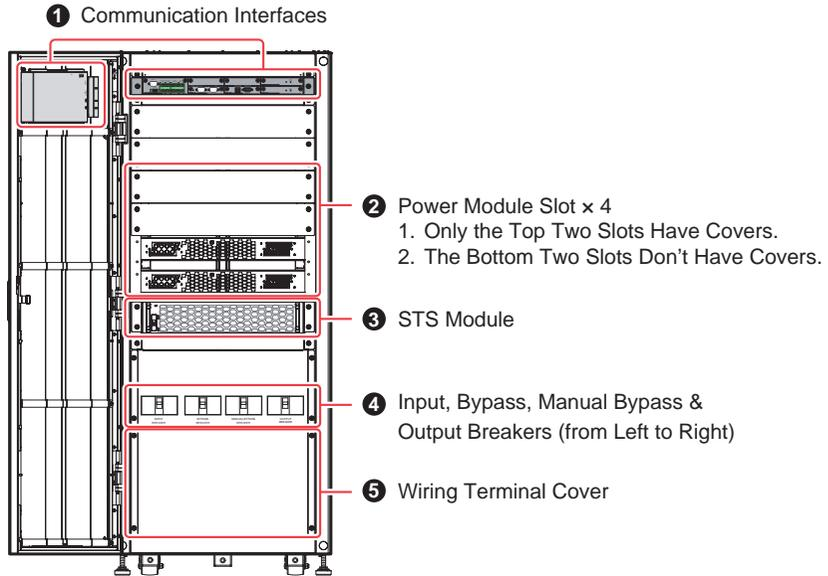
**(20 ~ 120kVA UPS Internal View with Front Door Open)**
