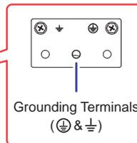
(Figure 2-10: Wiring Terminals\_ Grounding)
