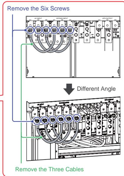
(Figure 5-7: Remove the Six Screws & Three Cables)
