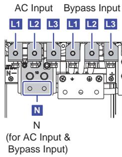
(Figure 2-7: Wiring Terminals\_ AC Input & Bypass Input)
