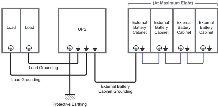
(Figure 5-16: Grounding Diagram\_ Single Unit)
