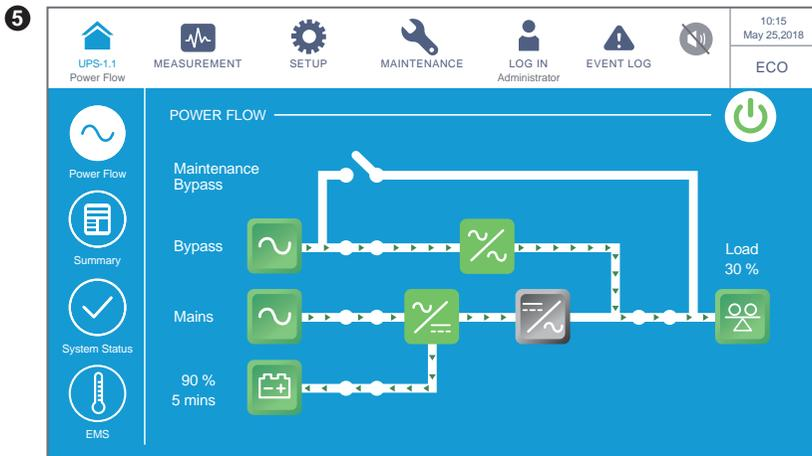
The screen above indicates that the UPS is in **ECO** mode. The inverter is in the ready-to-power-on status, and the power supply of the loads comes from the bypass. For **ECO** mode settings, please refer to **7.10.2 Mode Setting** and **6.2.5 ECO Mode Start-up Procedures**.
