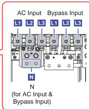
(Figure 5-8: Wiring Terminals\_ AC Input & Bypass Input)
