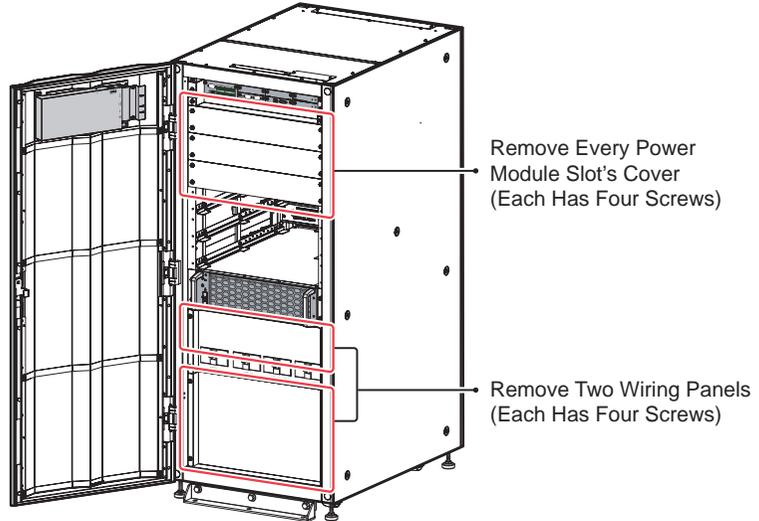
(Figure 4-21: Remove Every Power Module Slot's Cover and Wiring Panels)
