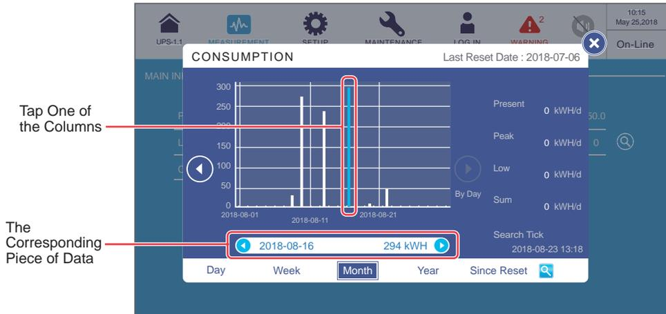
(1) Take the figure above as an example; if you tap the column '2018-08-16', the data bar that shows the corresponding piece of data will appear below the chart and show the UPS's main input kWH statistics '294kWH' of the day.
