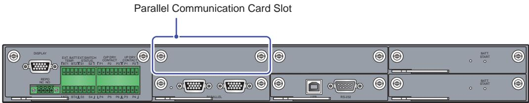
(Figure 4-12: Location of Parallel Communication Card Slot)
