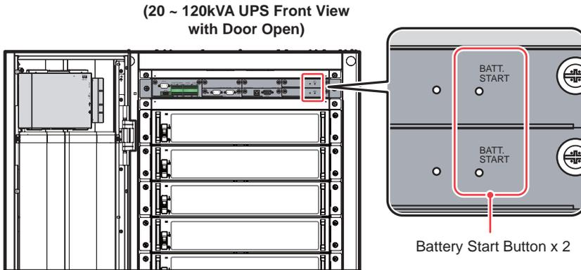
(Figure 7-2: The Position of Battery Start Buttons)
