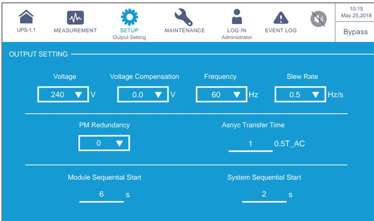
The screenshot shows the 'OUTPUT SETTING' screen with the following parameters:
