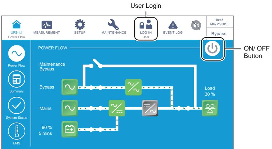
(Figure 7-5: Main Screen\_ User Login & ON/ OFF Button Location)
