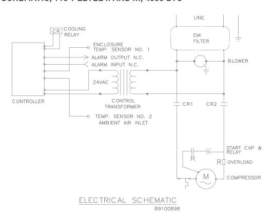
NOTE: For voltage, hertz, and options not shown in this manual, refer to the wiring diagram attached to the unit.
