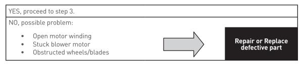
3. Check thermostat setting and adjust thermostat to the lowest setting. This should turn on the condenser blower and compressor. Did condenser blower and compressor come on when the thermostat was turned on?
